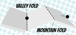
Folding is important. Dash lines represent mountain folds and should be folded downwards or away from you. Dot-dash lines represent valley folds and should be folded upwards or towards you. Fold the pieces according to their type of fold.
